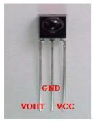
Infrared receiver has 3 pins.When you use it, connect VOUT to analog pin, GND to GND, VCC to +5V.Infrared remote control experiment
