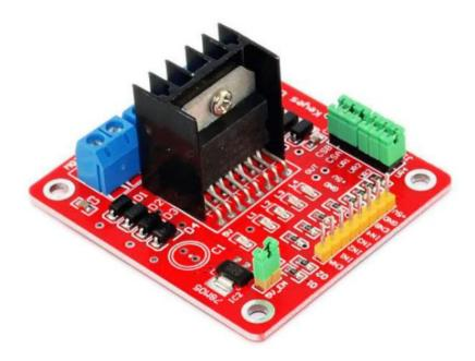
Double H driver module uses ST L298N dual full-bridge driver, an integrated monolithic circuit in a 15- lead Multiwatt and PowerSO20 packages. It is a high voltage, high current dual full-bridge driver designed to accept standard TTL logic levels and drive inductive loads such as relays, solenoids, DC and stepping motors.
