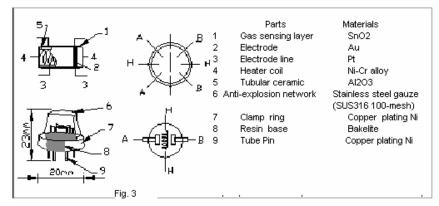
Structure and configuration of MQ136 gas sensor is shown as Fig. 3, sensor composed by micro AL2O3 ceramic tube, Tin Dioxide (SnO2) sensitive layer, measuring electrode and heater are fixed into a crust made by plastic and stainless steel net. The heater provides necessary work conditions for work of sensitive components. The enveloped MQ-4 have 6 pin, 4 of them are used to fetch signals, and other 2 are used for providing heating current.
