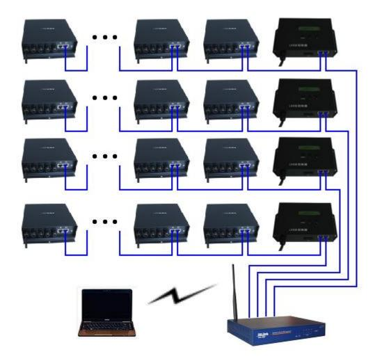
(4). Using optical fiber to acquire further transmission distance. If slave control to slave control requires the use of optical fiber, you need to add a IP converter, the use of specific methods please refer to the slave control instructions.
