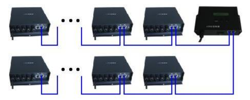
(2). Work online, H803TC transmit data from computer to slave controller, if there is no data sent from computer, H803TC will read data from SD card and send it to slave controller automatically.
