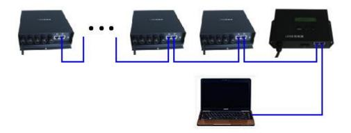
(3). Use switch to output to multiple network interfaces, the following picture illustrates the process: computer's wireless network card send data to wireless switch, and then transmit data to H803TC, you can also use the cable network card to send data, data is received by several H803TCs, the following picture only draws four H803TC receivers, you can use more according to actual needs.
