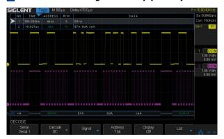
SDS1000X displays the decoding through the events list. Bus protocol information can be quickly and intuitively displayed in table form
