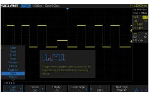
SDS1000X has a wealth of trigger modes, including Edge, Slope, Pulse, Video, Windows, Runt, Interval, Time out (Dropout), Pattern, IIC, SPI, UART/RS232, LIN, CAN
