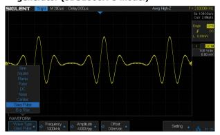
The SDS1000X-S has a built-in 25MHz function / arbitrary waveform generator, including 10 built-in waveforms plus 4 ARBs. The EasyWave PC software (included) to enter and edit arbitrary waveforms
