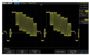
SPO display technology provides for fast refresh rates. The resulting intensity-graded trace is brighter for more often-occurring display points and dimmer in less-often-occurring points
